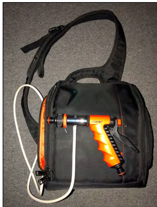
SG-OzPak exterior view of the backpack showing the JetSpray gun
