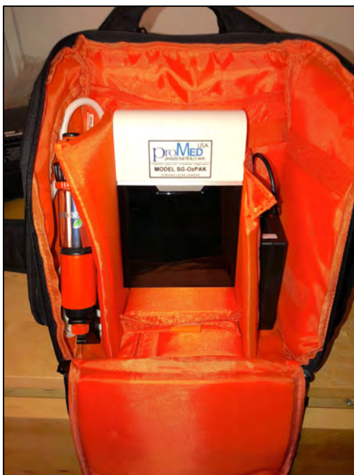
SG-OzPak interior view showing the battery pack and the Ozone Generator
