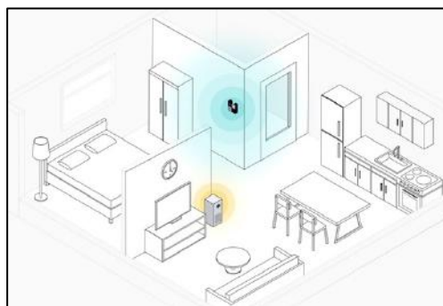
Area covered by built-in sensors in an air purifier vs an Atmocube IAQ monitor
